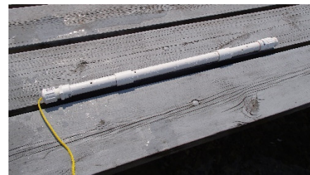
Figure 2. Example of a peeper with sample chambers at each capped end
