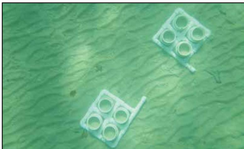
Equipment installed on the lake floor. This experiment is intended to determine to what extent nutrients in groundwater seeping up into the lake floor influence the GBA growth.
