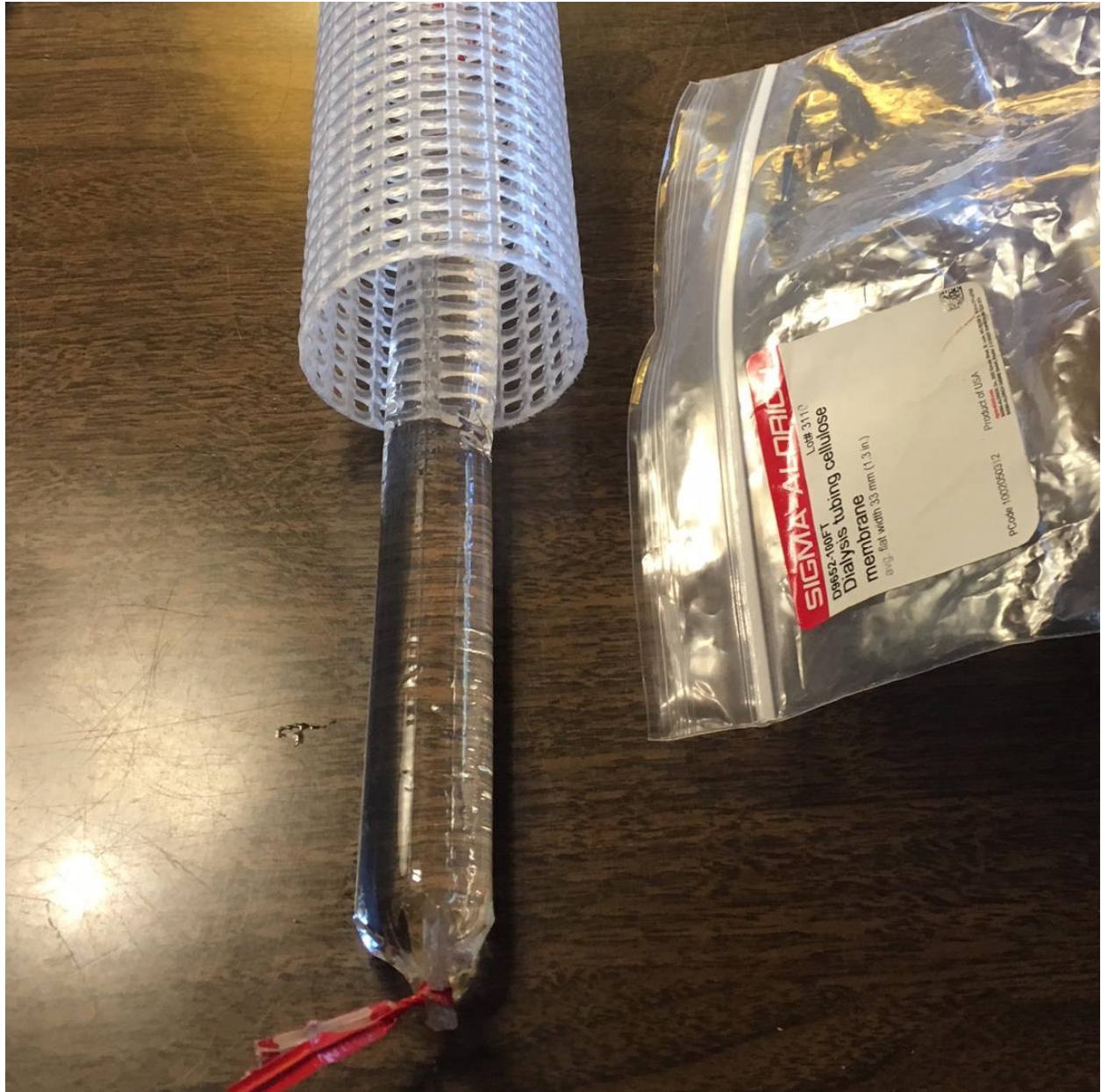
Figure 1. Dialysis tubing baggie and rigid mesh tube housing
