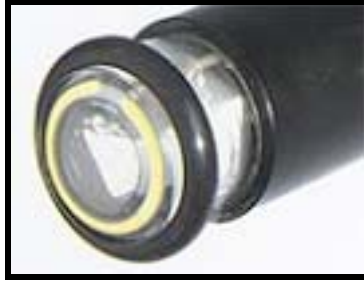
Hydrolab dissolved oxygen sensor
